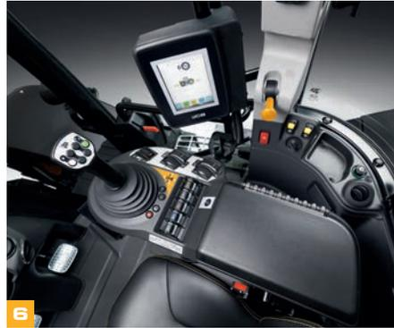
7 Seat-mounted console houses the most frequently used control switches and dials with a generously padded armrest built in.
