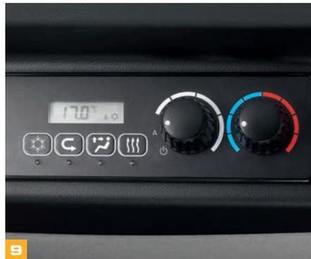
10 Climate control air conditioning keeps the temperature comfortable and quickly de-mists the windows on early mornings. Opening rear three-quarter windows add natural ventilation and a fixed roof window option floods the cab with light.
